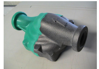
Depainting of expensive cast iron parts. The right hand side shows the surface with paint completely removed.
